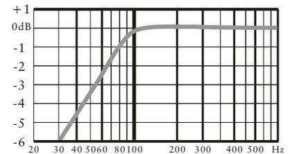
When LF cutting is at 25Hz, it equals discrete a 25Hz high pass filter on input circuit, it just attenuate the signal lower than 25Hz.
