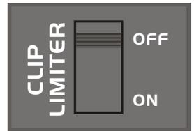
As the below drawing, when the switch is ON, the limit is on, if the input signal is too strong, the limit circuit can control the gain and reduce the distortion, also control the average output power, but it does not affect peak power, protect the loudspeaker and assure the dynamic of music.
